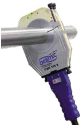
Due to their design, enclosed weld heads offer complete top layer protection of the weld joint due to continuous weld joint fluting during the welding process with protective gas. This reduces the joints' tempering colours.
